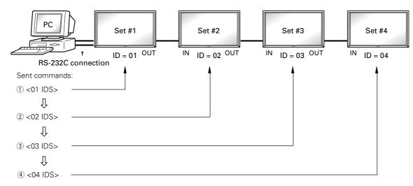
By sending RS-232C commands in this order, it is possible to assign an ID for each panel.
