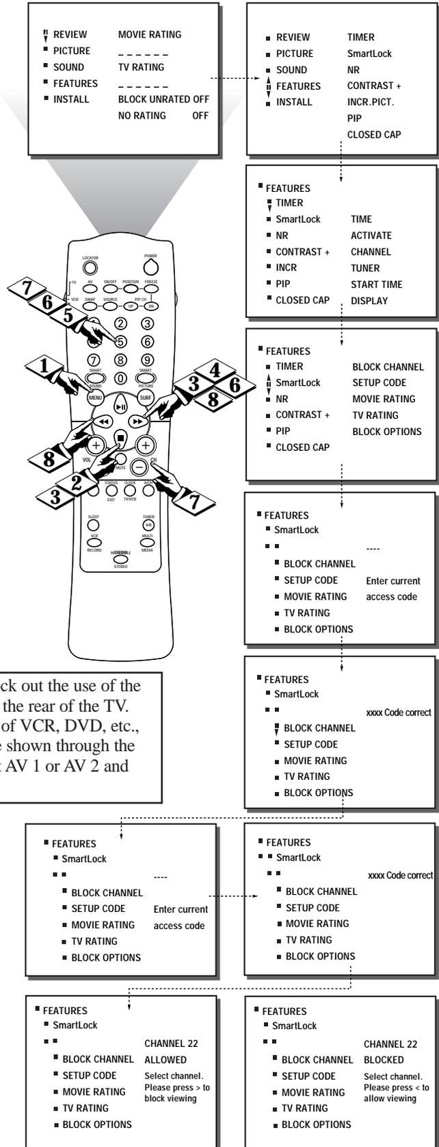
**Note:** You can also block out the use of the A/V external inputs on the rear of the TV. This stops the viewing of VCR, DVD, etc., programs which can be shown through the A/V Input jacks. Select AV 1 or AV 2 and select block.
