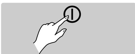
To switch on the set, press the on/off key. A red indicator comes on and the screen lights up. Go straight to the chapter Quick installation on page 4. If the television remains in standby mode, press on the remote control. The indicator will flash when you use the remote control.
