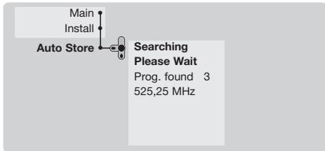
If the menu is not displayed, press and hold down the  $\Delta$ - and  $\nabla$ + keys on the TV set for 5 seconds to start the tuning (or MENU key depending on versions).
