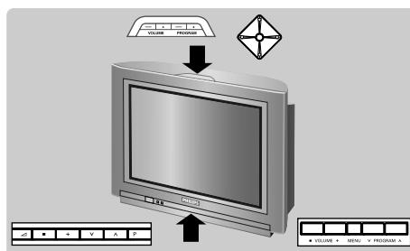
The VOLUME - (- +) keys are used to adjust sound levels. The PROGRAM - + (- +) keys are used to select the required programmes. To access the menus, simultaneously hold down the and + keys (or MENU key). The PROGRAM - + keys may then be used to select an adjustment and the - + keys to make that adjustment. To exit from the menus, hold down the 2 and + keys (or MENU key). Note : when the **Child Lock** function is activated, these keys are unavailable (refer to **Features** menu on page 7).
