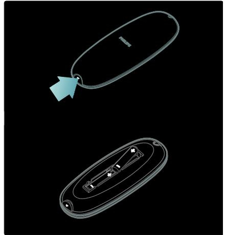
**Note:** The location of the battery compartment on some remote controls may be as follows:
