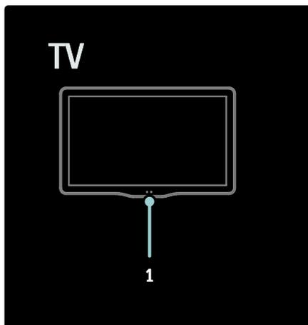
1. Ambient sensor/ remote control sensor.
