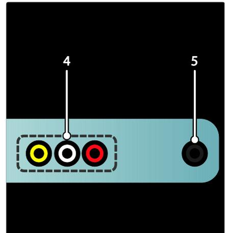
4. **AV IN :** Analog audio and video input from analog or digital devices such as DVD players, satellite receivers and VCRs.
