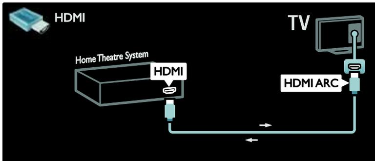
HDMI ARC allows you to use Philips EasyLink to output TV audio directly to a connected audio device, without the need for an additional digital audio cable. Be sure that the device is HDMI-CEC and ARC compliant, and that the TV is connected to the device using a HDMI cable attached to HDMI ARC connectors.
