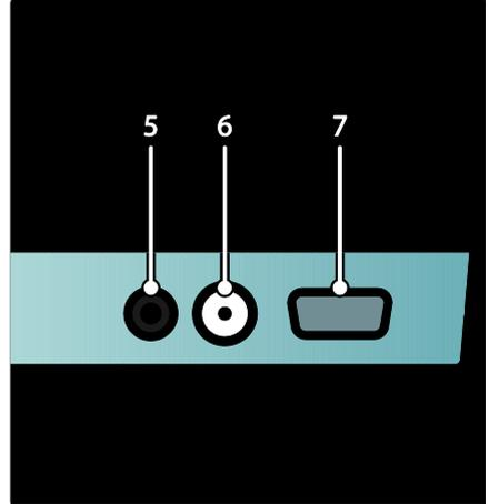
5. **AUDIO IN**: Audio input from devices that require a separate audio connection, such as a computer.
