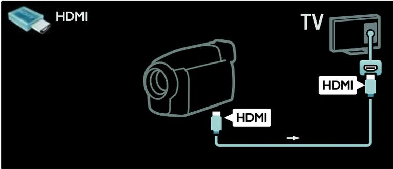
Otherwise, use an HDMI or the component video and audio cable (YPbPr and Audio L/R) to connect the camcorder to the back of the TV.
