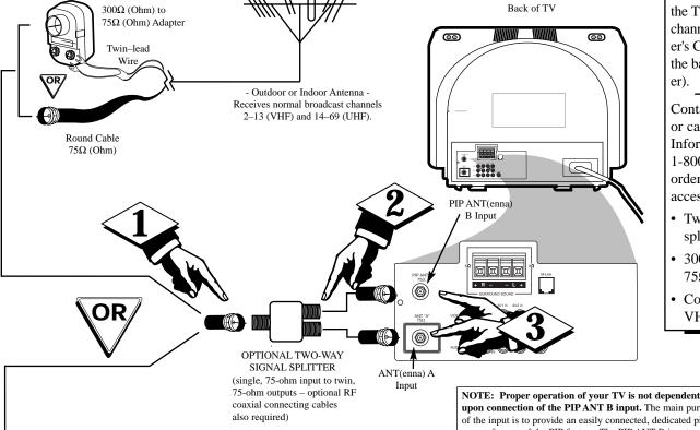
upon connection of the PIP ANT B input. The main purpose of the input is to provide an easily connected, dedicated picture source for use of the PIP feature. The PIP ANT B input can, however, be used to connect and display other signal source options such as a satellite dish system, an additional external antenna, a VCR, or a video game, for example
