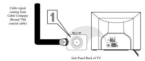
Cable Box with RF Inputs and Outputs Connection:
