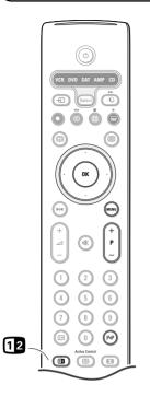
Press the 12 key to switch on Dual screen, **PIP** or one of the PIP modes.
