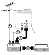
Connect the aerial cables (1), (2) and, to obtain the optimum picture quality, eurocable (3) as shown.
