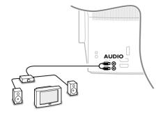
To enhance the sound reproduction of your TV you can connect two extra front loudspeakers via an external amplifier.
