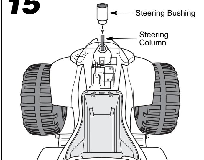
**Helpful Hint:** You may want the help of another adult to support the steering column near the steering linkage while assembling the handlebar to the vehicle body.
