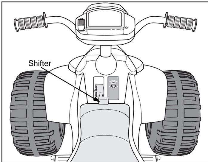
**Please Note: To avoid damaging the motors and gears, make sure to stop the vehicle before switching from drive to reverse.**
