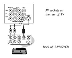
The S-Video connection on the rear of the TV is used for the playback of S-VHS VCR tapes, Video Discs, Video Games or Compact Disc-Interactive (cd-i) discs. Better picture detail and clarity is possible with the S-Video playback as compared to the picture from a normal antenna (RF) connection.
