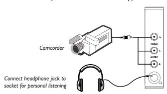
For more convenient direct playback connections, the Side Audio/Video Input sockets allow for quick and easy connections, particularly Camcorder tape recordings.
