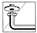
To fit the stand remove the feet on the TV using the key supplied (see illustration).
