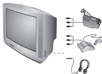
Depending on the versions, the connectors are located on the front (sometimes under a flap) or on the right-hand side of the TV set. Make the connections as shown opposite. With the **AV** key, select AV.
