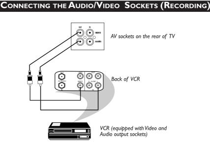
Connect the sockets of the VCR which you wish to record from, to the corresponding AV sockets.
