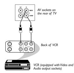
You can view the playback of VCR tapes (Video Disc players, camcorders, etc.) by using the AUDIO and VIDEO INPUT sockets on the rear of the TV.
