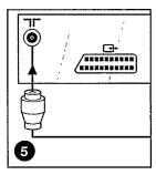
If the TF socket is used then the signal must be stored on a program number before it can be selected (refer to the section 'to store the video recorder signal on a program number').
