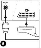
A device with a Euroconnector can be connected to the Euroconnector socket located at the back of the TV (a support bracket is provided for the Euroconnector cable on the back of the TV).
