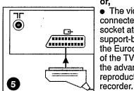
or, • The video recorder can also be connected at the Euroconnector socket at the back of the TV (a support-bracket is also provided for the Euroconnector cable on the back of the TV). The Euroconnector gives the advantage of stereo sound reproduction from a suitable video
