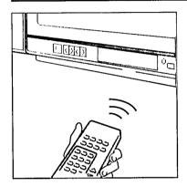
to select TV stations using program numbers to change the picture and sound settings to select protected switch-on mode to select stand-by mode to select the sound system (STEREO, DUAL, SPATIAL) to display picture and sound information
