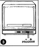
3. Select the required program number (0 to 39) by pressing the - or + PROGRAM button. The selected program number is displayed on the screen.
