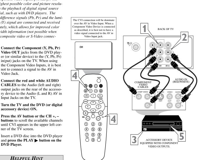
*Somponent Video inputs provide for the*  highest possible color and picture resolution in the playback of digital signal source material, such as with DVD players. The color difference signals (Pb, Pr) and the luminance (Y) signal are connected and received separately, which allows for improved color bandwidth information (not possible when using composite video or S-Video connections).
