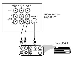
The S-Video connection on the rear of the TV is used for the playback of S-VHS VCR tapes, Video Discs, Video Games or Compact Disc-Interactive (cd-i) discs. Better picture detail and clarity is possible with the S-Video playback as compared to the picture from a normal antenna (RF) connection.
