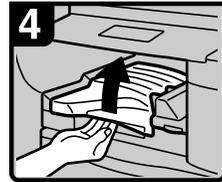
If you cannot remove the misfed paper, open the top cover of the bridge unit.
