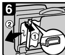
Pull the green lever in the upper left corner, and then remove the misfed original.
