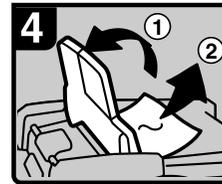
If you cannot remove the misfed original, open the ADF external cover, and then remove the misfed original.
