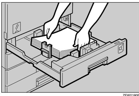
**7** While pressing the release lever, adjust the side guides to the new paper size.
