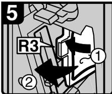
Open lever R3 to the left, and then remove the misfed paper.
