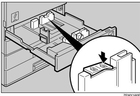
**5** While pressing the release lever, adjust the side guides.
