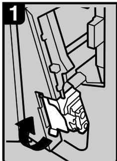
Open the front cover of the finisher, and then pull out the staple unit.
