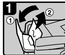
Open the cover of the auto document feeder (ADF), and then remove the misfed original.
