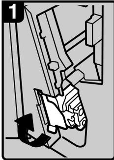
Open the front cover of the finisher, and then pull out the staple unit.
