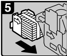
Align the arrows on the new refill with those on the cartridge, and then push in the refill until it clicks.
