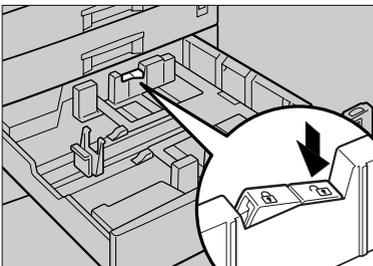
**5** While pressing the release lever, adjust the side fences.
