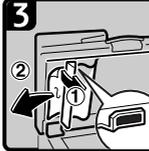
3. Pull the green lever in the upper left corner, and then remove the misfed original.
