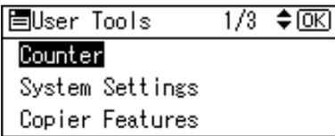
**3** Select **[Key Operator Tools]** using **[▲]** or **[▼]**, and then press the **[OK]** key.
