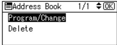
**6** Enter the registration number you want to program using the number keys or the Quick Dial keys, and then press the **[OK]** key.
