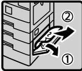
1. Open the lower right cover of the optional paper tray unit and remove the misfed paper.
