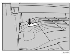
Pushing in the Output Tray Guide Push in the Output Tray Guide.
