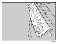
**1** To tilt the control panel downwards, press the adjustment button to unlock the panel, and then gently adjust it until it locks into position.
