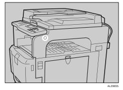
**2** Tilt the control panel upwards, and then release the adjustment button to lock the panel.
