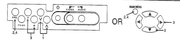
Cancelling previously adjusted (manually) fine tuning, means reactivating the AFC (Automatic Frequency Control) Function, also known as AFT (Automatic Frequency Tuning). Reactivating the Automatic Fine Tuning means allowing the set to automatically tune optimum tuning position, for that Channel Number.
