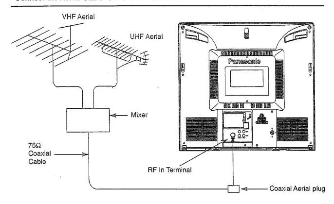
To obtain the best quality picture and sound, an external antenna, the correct cables (75 Ohm coaxial) and the correct terminating plug will be required.
