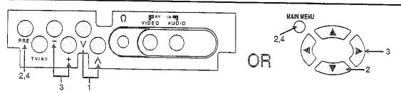
Under normal reception condition, this function is not used. However, in areas of poor reception or constant interference, a slight adjustment on the fine tuning can improve the picture and sound quality.
