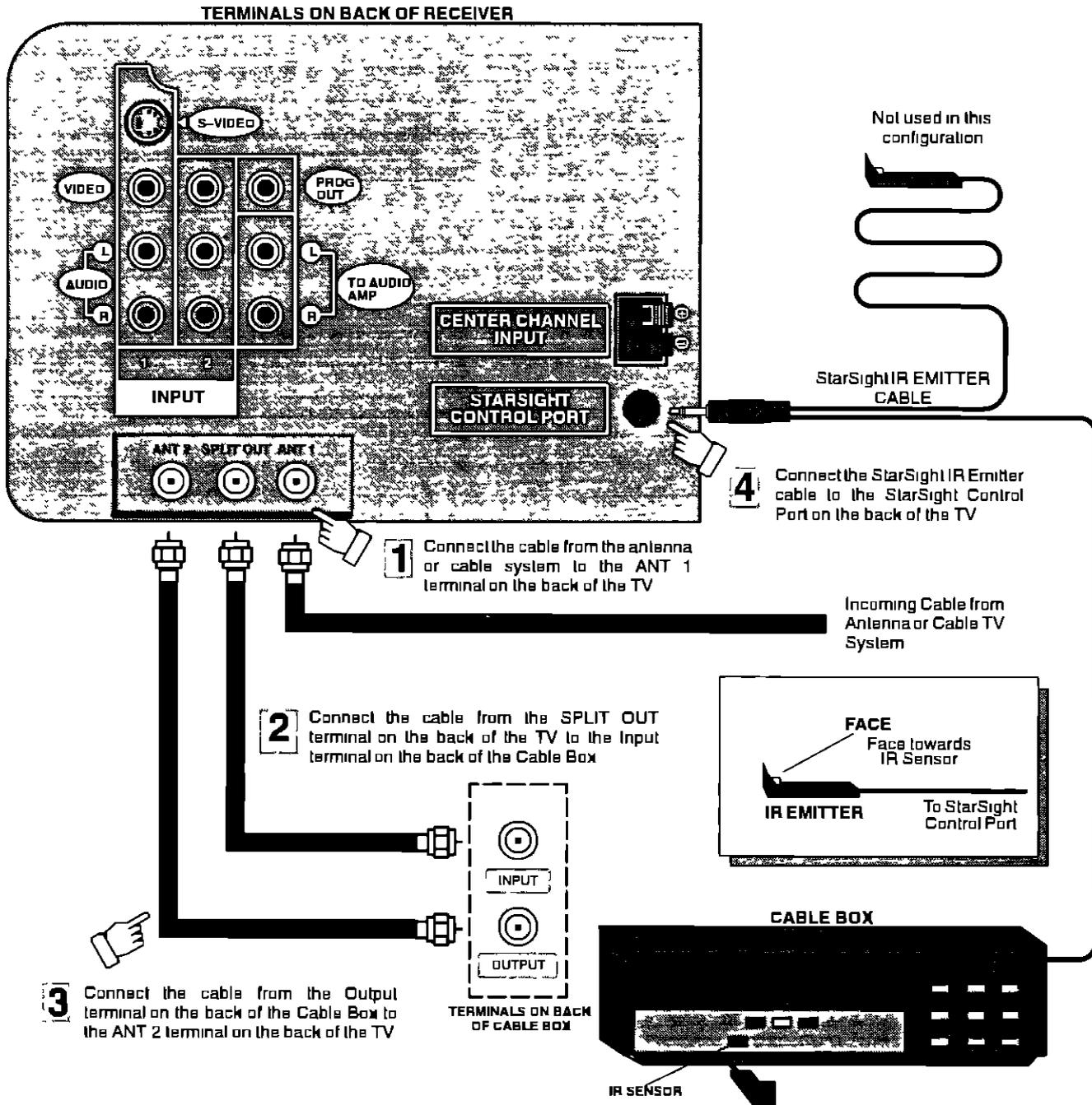
**3** Connect the cable from the Output terminal on the back of the Cable Box to the ANT 2 terminal on the back of the TV
