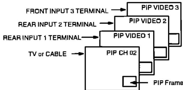
**PIP (Picture in Picture) Button** – This feature allows the viewer to monitor one channel program while watching another. The monitored source (PIP) can be a different channel or a different video source (such as a VCR) when connected to the input jacks
