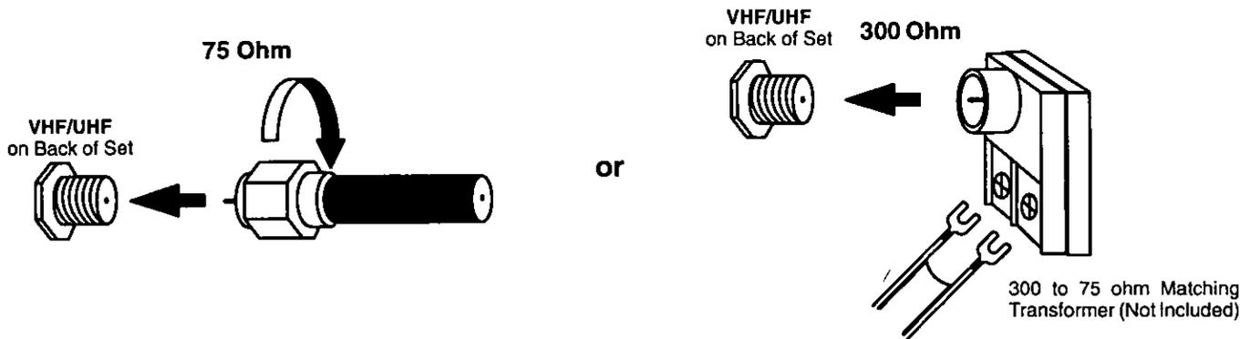
**Cable Connection** – For reception of cable channels, connect the cable supplied by your local cable company. In the **SETUP** menu, set the **MODE** to **CABLE**. (Refer to Antenna Mode section.)
