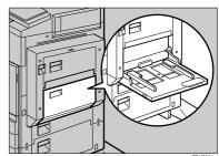
Insert the paper with the side you want to copy facing down until you hear the beep, and align the paper guide to the paper size.
