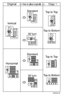
This table shows the orientation of images on the front and back of copies, not the orientation of delivered copies.
