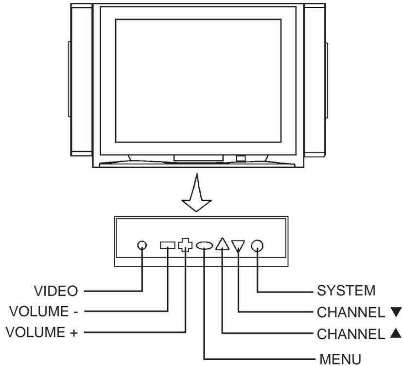
Note: Functions of
