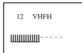
↓ After presetting is finished it returns to the first channel
