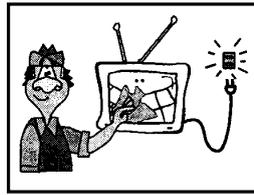
In order to wipe dust off the picture tube or off the cabinet, you should remove the power plug from the wall outlet first. You can wipe lightly with a piece of dry, clean, soft cloth.
