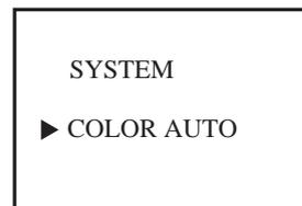
6.2 If the displaying colour is abnormal, press the ▼ or ▲ button to select COLOUR, then press the → or ← button to select the right colour system. Every time you press → or ← button, the colour system will change in the sequence on the right.
