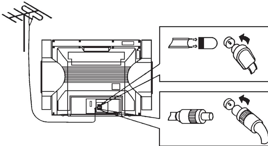
Note: In case of using the Twin-lead aerial feeder ( $300\Omega$ ) for UHF/VHF aerial, use a 300-75 ohm adaptor (not supplied)
