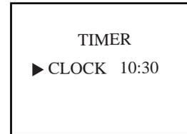
**Note: To make use of ON TIME and OFF TIME, set the clock firstly and check the correct time.**
