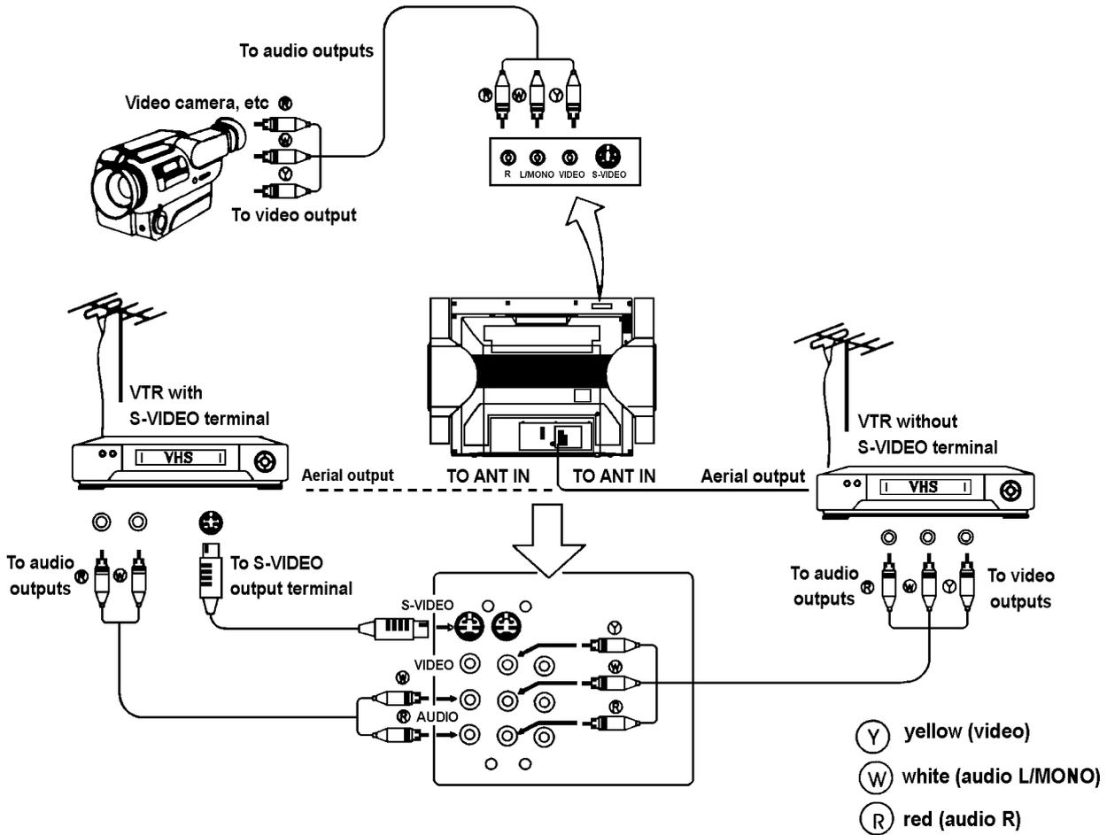
To select the input press the VIDEO button on the TV set or the AV button on the remote controller repeatedly until you see the corresponding input indication on the screen. To return to aerial input, press the AV button until it displays programme number, or press direct channel select button or the CH ▲/▼ button.
