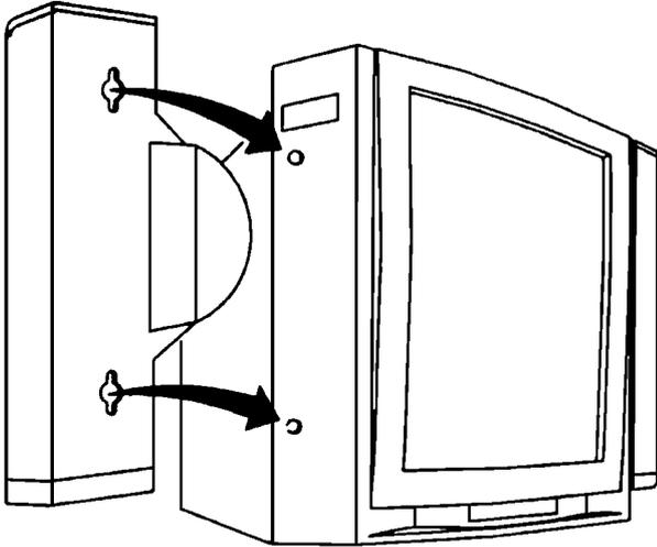
Loosen the screws to remove the speaker from the TV
