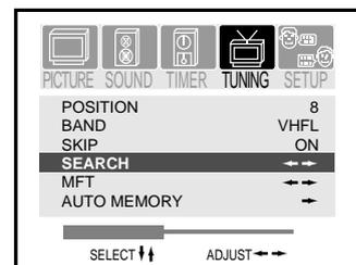
When searching towards higher frequency, pressing **VOL-** will stop the search and return to first program. When searching towards lower frequency, pressing **VOL+** will stop the search and return to first program.
