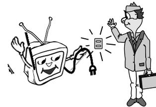
◆ Don't overload wall outlets; extension cords, or integral convenience receptacles as this can result in a risk of fire or electric shock.
