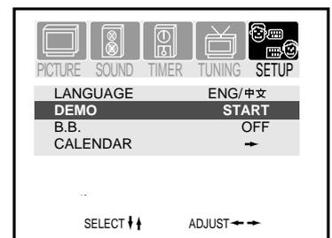
After the demonstration, it will return to **SETUP** menu and the **DEMO** item is auto set to **STOP**. After 4 seconds it exits the menu automatically.
