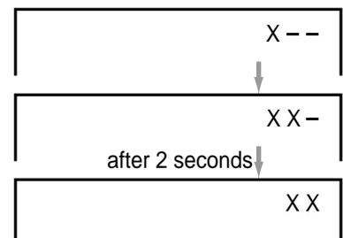
**Method 2:** press 0 button, and then input the channel number. Be sure the period of two-press should be within 2 seconds.
