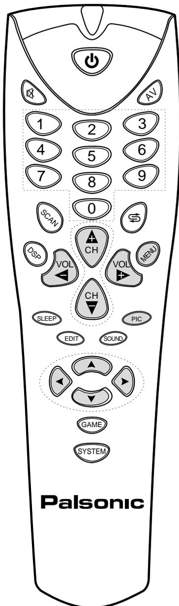
**5** Press **VOL+** to search towards higher frequency, the screen displays glittering "→" press **VOL-** to search toward lower frequency, the screen displays glittering "←". When a channel is located, the searching stops and the channel is stored in the specified channel number.
