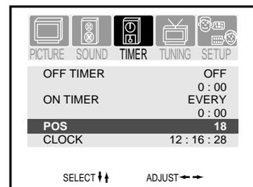
If the set is in standby mode, it will auto turn on and broadcast the preset channel at the preset time. If in normal working mode, the set will auto switch to the preset channel at the preset time.
