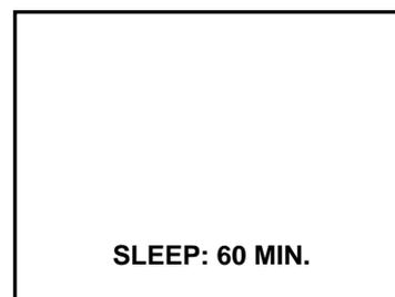
For example, you would like the TV to turn off in 60 minutes, you can press the **SLEEP** button repeatedly until the screen displays **60 MIN.**
