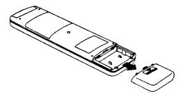
2) Insert two size AAA batteries according to the polarity indication inside the remote controller.
