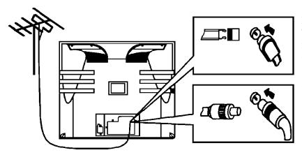
Note: In case of using the Twin-lead aerial feeder (300 $\Omega$ ) for UHF/VHF aerial, use a 300-75 ohm adaptor (not supplied)
