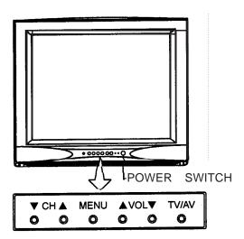
Note: Functions of ▲ CH ▼, MENU, ▲ VOL ▼, TV/AV are also provided to the remote controller.
