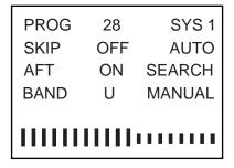
Making use of the **PRESET** menu can fulfil the function of auto-search, search. manual search, channel and band selection. AFT and skip on/off.
