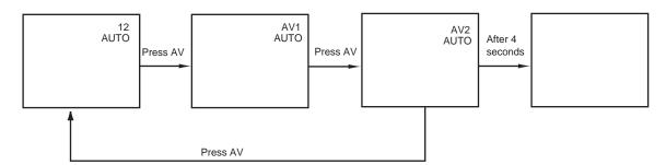
Note: S-VHS IN and AV2 use the same interface. If you want to receive signals input through S-VHS terminal, switch the set to AV2, the S-VHS (S-VIDEO) input terminal has priority over the AV2 VIDEO terminal; To use equipment connected to the AV2 VIDEO IN terminal, disconnect any plug from the S-VHS terminal. S-VHS and AV2 use the same group of AUDIO IN terminals.
