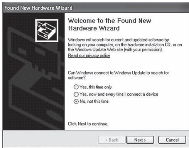
Figure 5a. When initially connecting the SSDSI-II to a Windows XP computer, the Found New Hardware Wizard will appear and guide you through driver installation.
