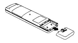
Insert two size AAA batteries according to the polarity indication inside the remote controller.
