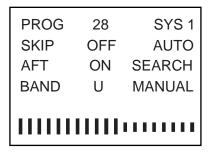
Making use of the **PRESET** menu can fulfil the function of auto-search, search. manual search, channel and band selection. AFT and skip on/off.
