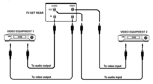
Press AV button on the remote control unit to select AV mode before dubbing, "AV" will be displayed on the screen. The TV set will act as a monitor to help you edit while dubbing. NOTE: The set MUST remain in Video mode and MUST NOT be switched off during the session.
