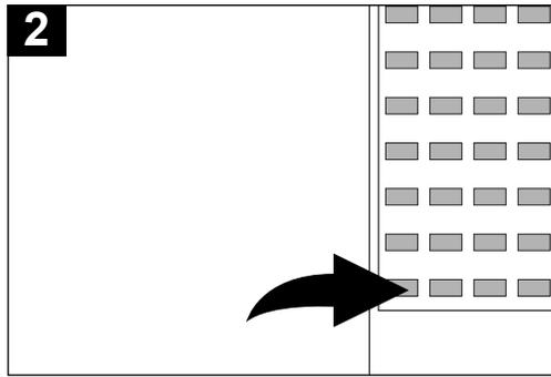
2 Simply press the TV/CATV button to set the TV to TV or CATV (Cable TV) mode. To change the type of cable (STD, HRC, IRC), simply change the TV/CATV option under the TUNING menu.
