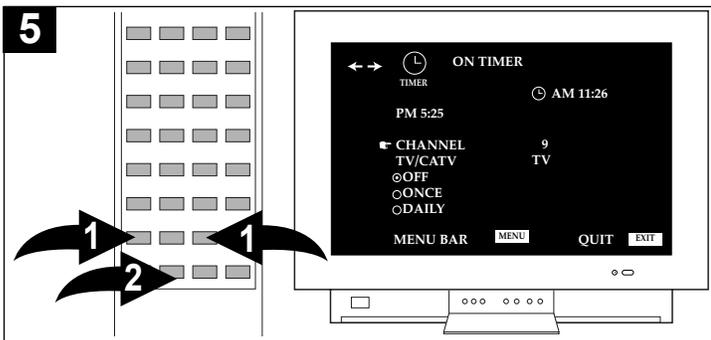
Press the Navigation (▼) button ❷ and then the Navigation (◀) and (▶) buttons ❶ to set the desired channel you would like the TV to turn on to.
