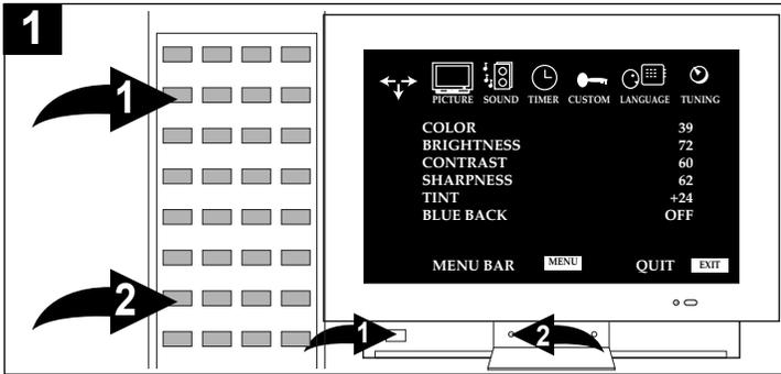
Press the POWER button ❶ to turn on the TV. Press the MENU button ❷; the MENU screen will appear.
