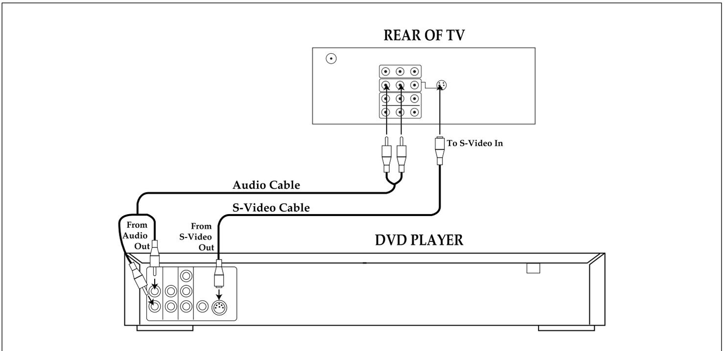
1. Connect the left and right audio cable from the DVD's Audio OUT jacks to the TV's AV1 left and right Audio IN jacks.
