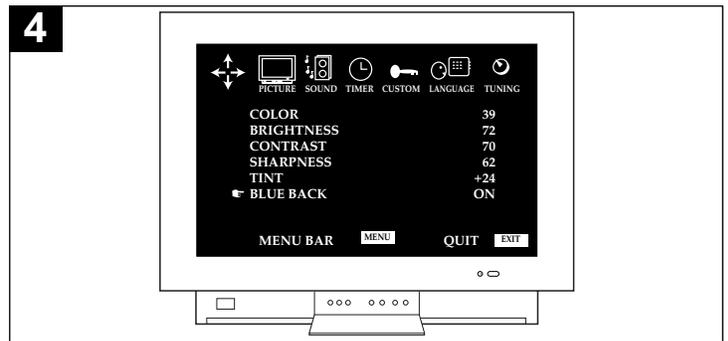
If the Blue Back option is set to ON, when a station is selected with no broadcast signal, a blue screen will appear. Turn this option off if using a DVD player.
