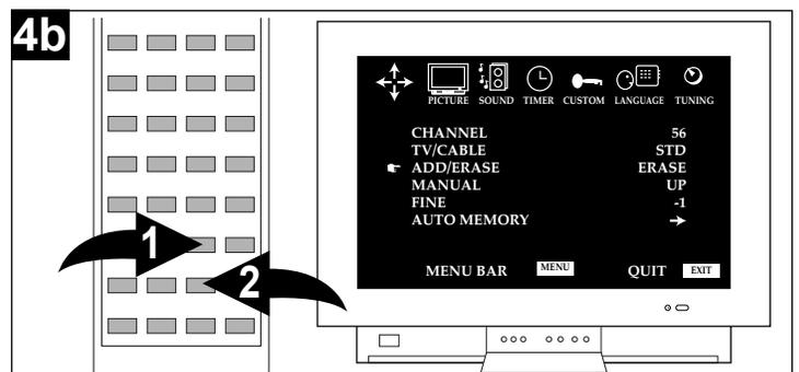
When a channel is selected and ADD appears next to the ADD/ERASE option, press the Navigation (▶) button ❷ to erase the channel. Press the EXIT button ❶ to exit the Tuning screen.
