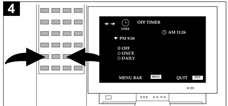
Using the Navigation (◀) and (▶) buttons, set the desired time you would like the TV to turn off (make sure to set the correct AM/PM). Press and hold either button and the time will increase/decrease in 10 minute increments.
