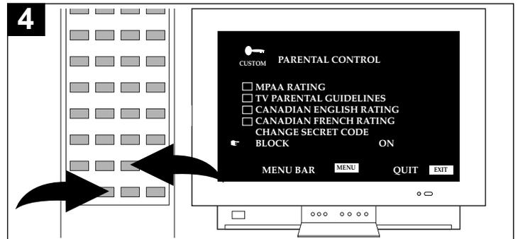
Scroll down to BLOCK using the Navigation (▼) button. When BLOCK is red, press the Navigation (▶) button to turn it on or off.
