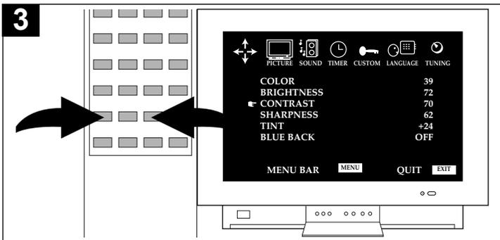
Adjust the setting using the Navigation (◀) and (▶) buttons as desired.
