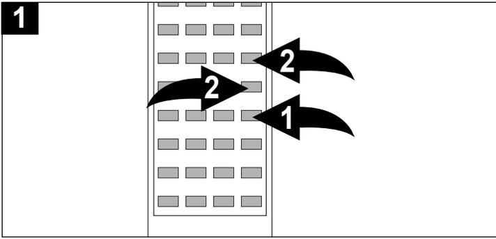
Press the MUTE button ❶ to turn off the sound. The TV's sound will be silenced and "MUTE" will appear on the screen. The sound can be turned back on by pressing this button again or one of the VOLUME + or - buttons ❷.
