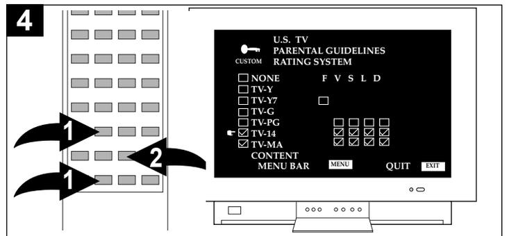
Using the Navigation (▼) or (▲) button ①, select the desired rating, then press the Navigation (▶) button ②. The letters/boxes next to the ratings represent the following:
