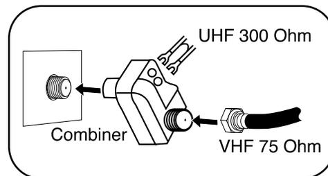
Connect the 75 ohm cable from the VHF antenna and the UHF antenna twin-lead wire to a combiner (NOT SUPPLIED). Attach the combiner to the antenna jack.
