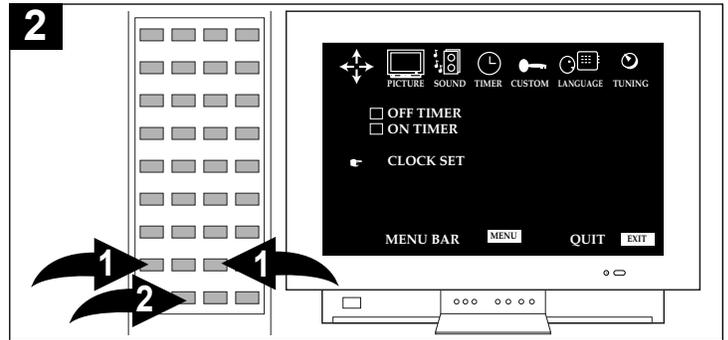
Press the Navigation (◀) or (▶) button ❶ until TIMER is selected, then scroll down using the Navigation (▼) button ❷ and select CLOCK SET.
