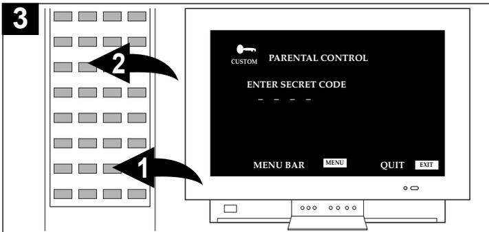
When PARENTAL CONTROL is in red, press the Navigation (▶) button ❶ to select it. Using the Direct Channel Selection buttons (0-9) ❷, enter the password ("0000" is the preset password if you have not changed it). This password can be changed to consist of different numbers (i.e. 1467, 9732) after the original password is entered.
