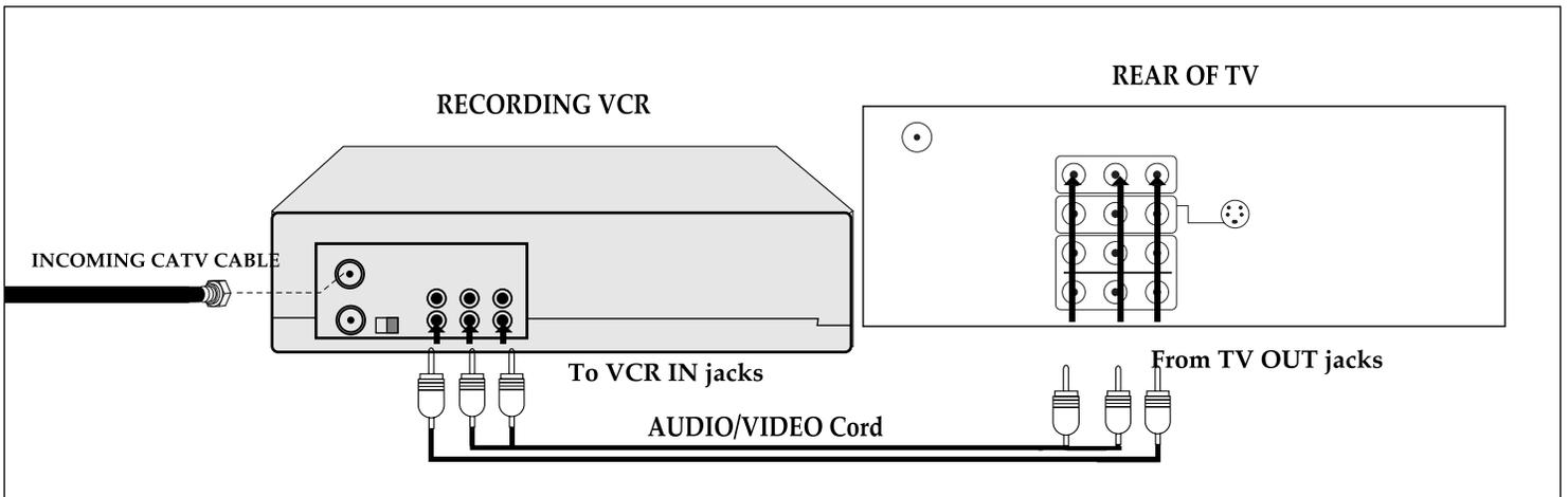
1. Connect the left and right audio cable from the TV's Audio OUT jacks to the VCR's left and right Audio IN jacks. Connect the TV's video OUT jack to the VCR's video IN jack.
