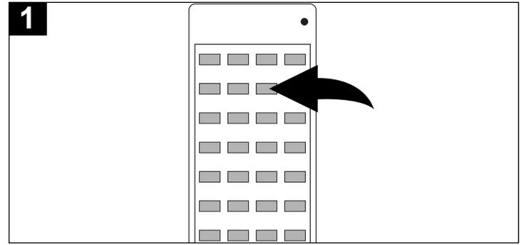
To set the TV to turn off after a preset amount of time, press the SLEEP button on the remote, "SLEEP:OFF" will appear on the screen. Each additional press will decrease the Sleep time by 10 minutes, from 120 minutes to 90 minutes. To confirm remaining sleep time, press the SLEEP button; the remaining time will briefly appear on the screen. To cancel the sleep time, press SLEEP button repeatedly until "SLEEP: OFF" appears on the screen.
