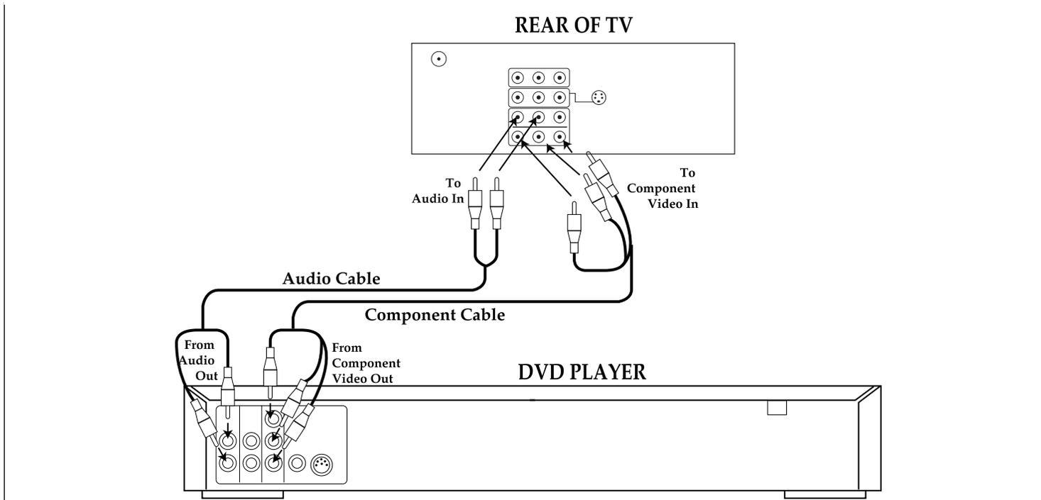
1. Connect the left and right audio cable from the DVD's Audio OUT jacks to the TV's AV2 left and right Audio IN jacks.
