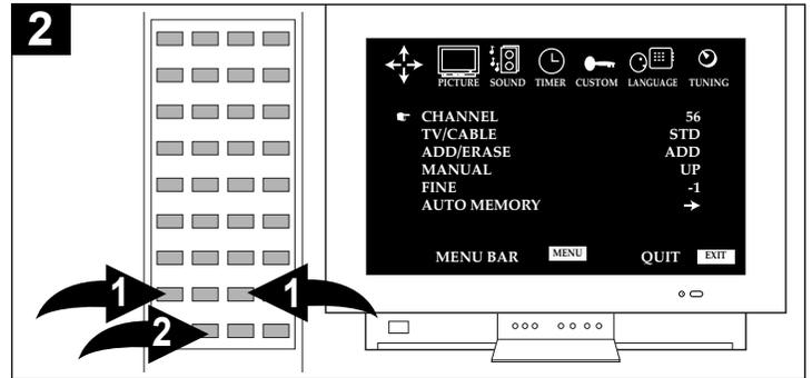
Press the Navigation (◀) or (▶) button ❶ until TUNING is selected, then scroll down using the Navigation (▼) button ❷ and select CHANNEL.
