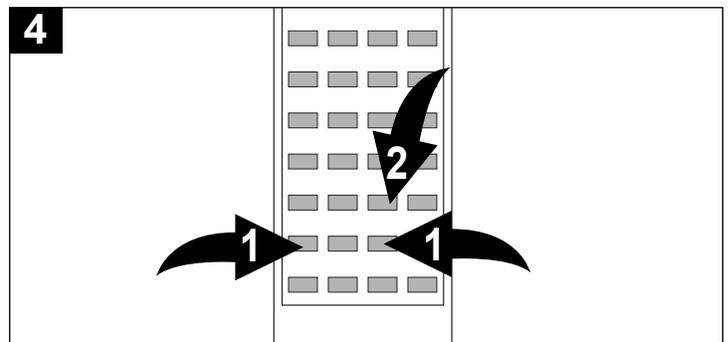
Using the Navigation (◀) and (▶) buttons ❶, set the correct time and AM/PM. Press and hold either button and the time will increase/decrease in 10 minute increments. Wait 15 seconds, or press the EXIT button ❸ to exit.
