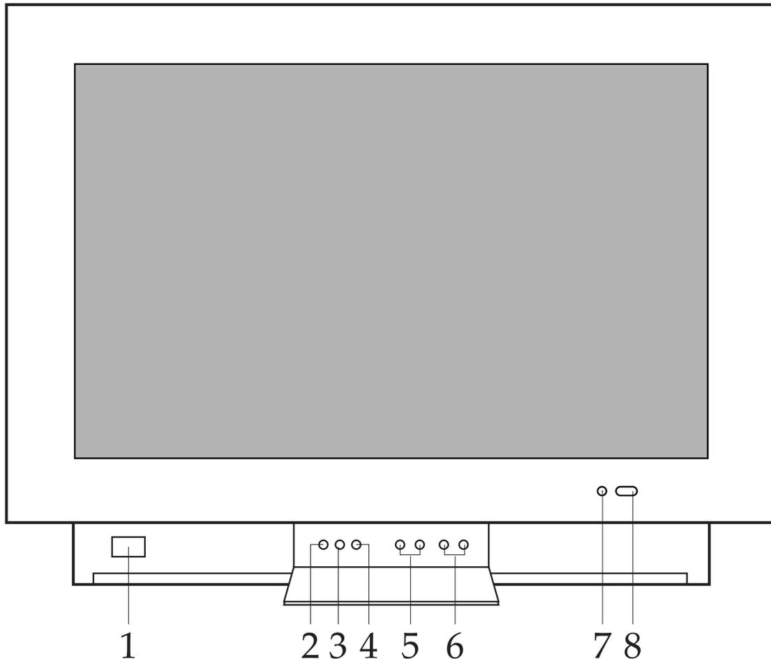
1. **POWER Button** - Press to turn the TV on; the Power indicator will light red. Press again to turn the TV off; the Power indicator will go off.
