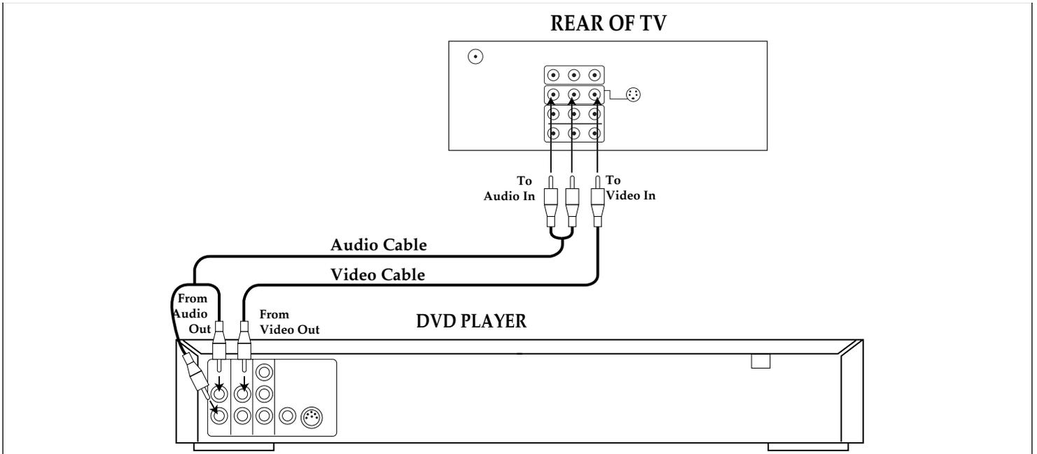
1. Connect the left and right audio cable from the DVD's Audio OUT jacks to the TV's AV1 or AV2 left and right Audio IN jacks. Connect the DVD's video OUT jack to the TV's video IN jack.
