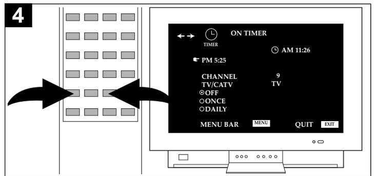
Using the Navigation (◀) and (▶) buttons, set the desired time you would like the TV to turn on (make sure to set the correct AM/PM). Press and hold either button and the time will increase/decrease in 10 minute increments.
