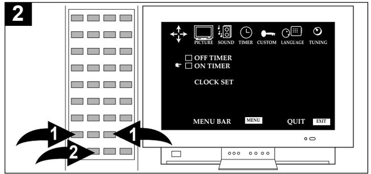
Press the Navigation (◀) or (▶) button ❶ until TIMER is selected, then scroll down using the Navigation (▼) button ❷ and select ON TIMER.
