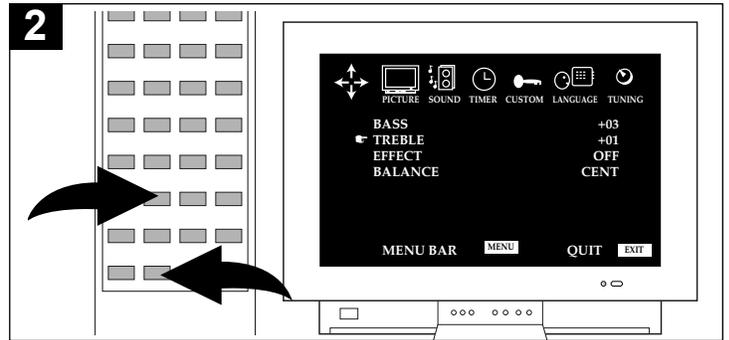
Press the Navigation (▲) or (▼) button to selected the desired sound setting (BASS, TREBLE, EFFECT and BALANCE).
