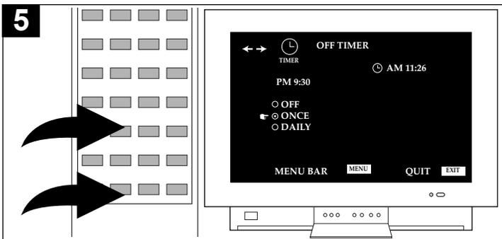
Press the Navigation (▲) or (▼) button to select between OFF (will turn Off Timer off), ONCE (will set the Off Timer to turn off once), or DAILY (will set the Off Timer to turn off Daily.)
