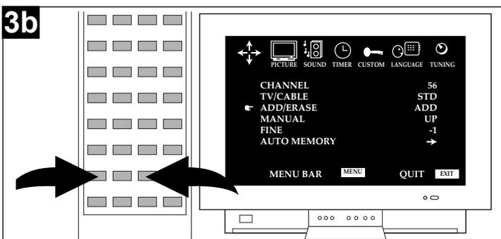
Press the Navigation (◀) or (▶) button to select a channel to be added. If a channel is already memorized, "ADD" will appear next to the ADD/ERASE option. If a channel is not memorized, "ERASE" will appear.
