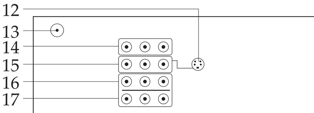
**12. S-VIDEO IN Jack (Rear of Unit)** - Connect an external unit that utilizes an S-video cable to this jack.
