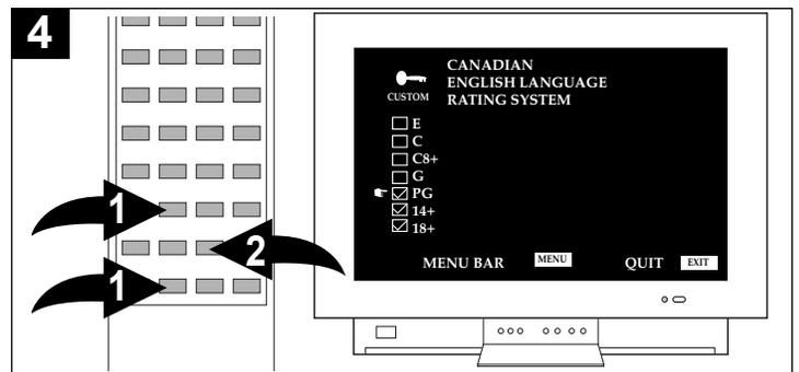
Using the Navigation (▼) or (▲) button ①, select the desired rating, then press the Navigation (▶) button ②. All programs with a higher rating than the one selected will also be blocked.
