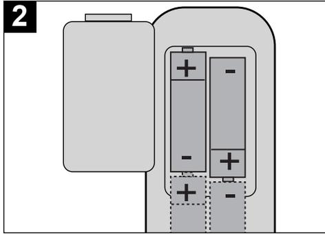
Install four "AAA" batteries, paying attention to the polarity diagram in the battery compartment.
