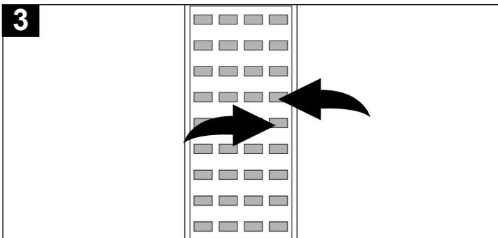
3 Adjust the volume level by pressing the VOLUME + or – button. The volume level will be indicated on the screen by green bars. As the volume level increases/decreases, so do the number of bars.
