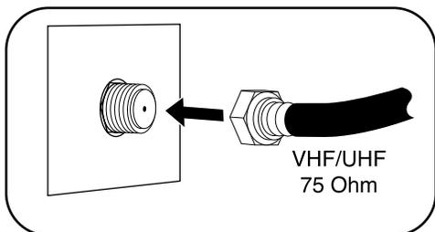
Connect the 75 ohm cable from combination VHF/UHF antenna to the antenna jack.
