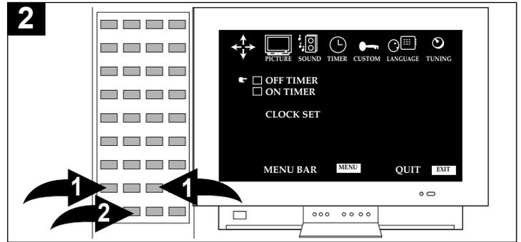
Press the Navigation (◀) or (▶) button ❶ until TIMER is selected, then scroll down using the Navigation (▼) button ❷ and select OFF TIMER.
