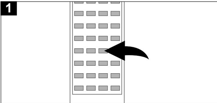
Press the RECALL button once, the channel being viewed and Stereo/Mono will appear.
