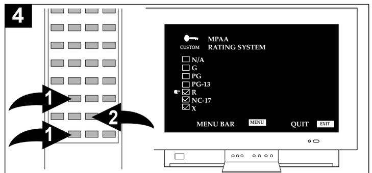
Using the Navigation (▼) or (▲) button ❶, select the desired rating, then press the Navigation (▶) button ❷. See below.
