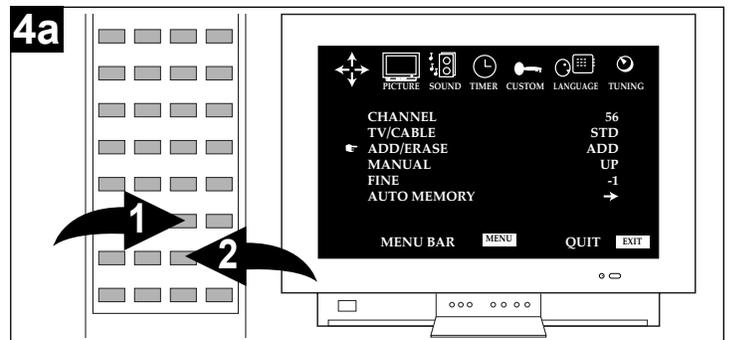
When a channel is selected and ERASE appears next to the ADD/ERASE option, press the Navigation (▶) button ❷ to add the channel. Press the EXIT button ❶ to exit the Tuning screen.
