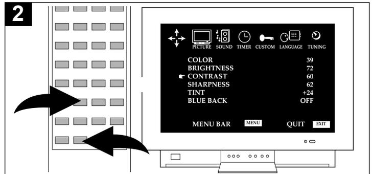
Press the Navigation (▲) or (▼) button to select the desired picture setting (COLOR, BRIGHTNESS, CONTRAST, SHARPNESS, TINT or BLUE BACK).
