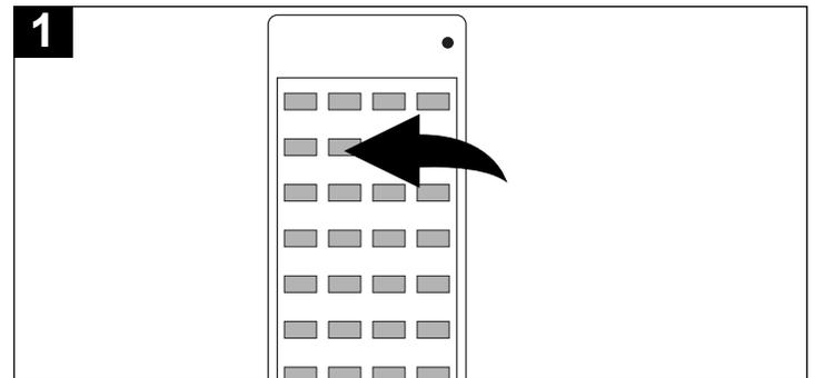
Press the AV button to cycle through the device(s) connected to the INPUT jacks; the jack number will appear on the screen. Repeatedly press to return to the antenna connected to the VHF/UHF IN jack (Cable TV, etc.).
