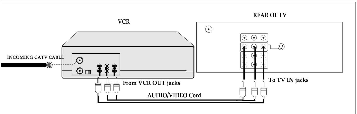
1. Connect the cable, satellite or incoming antenna to the ANT jack on the rear of the VCR.
