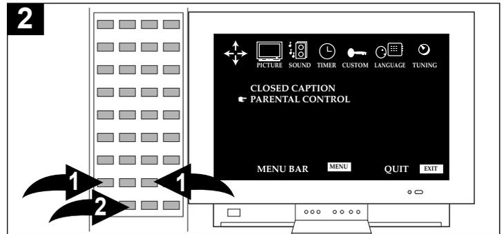
Press the Navigation (◀) or (▶) button ❶ until CUSTOM is selected, then scroll down using the Navigation (▼) button ❷ and select PARENTAL CONTROL.
