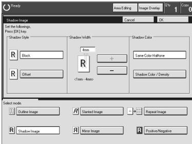
**4** Adjust the width by pressing the [+] or [-] key.
