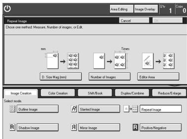
**5** Enter a horizontal and vertical number between 1 and 15, and then press the [#] key.
