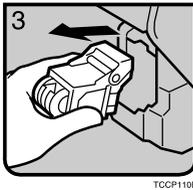
**4** Remove the empty refill in the arrow direction.
