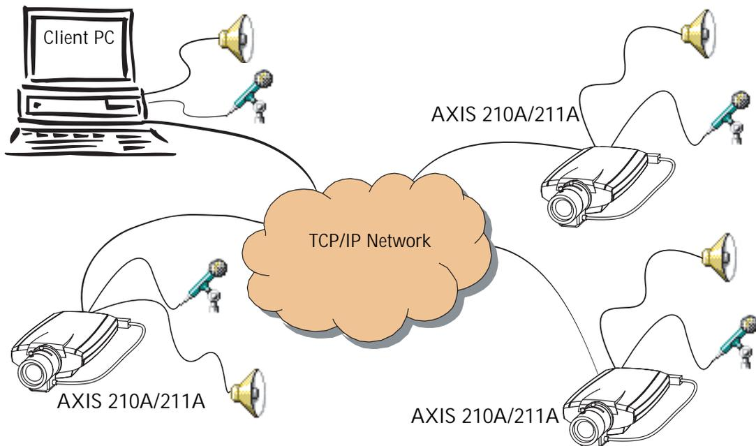
An example of a network using AXIS 210A/211A cameras to transmit audio and video across the network.
