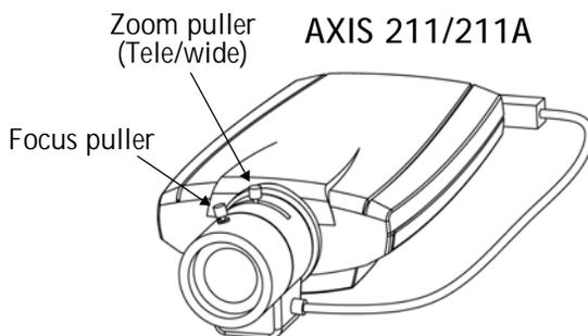
**Note:** The DC-Iris should always be disabled while focusing the camera. This opens the iris to its maximum, which gives the smallest depth of field and thus the best conditions for correct focusing. When the focus is set with this method it will then be maintained in any light conditions.
