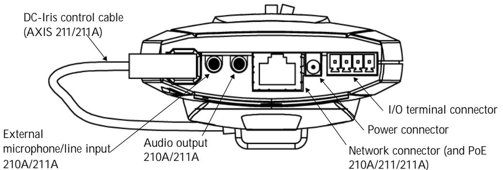
**Power Connector** - For connection of the PS-K power adapter (included).
