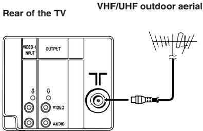
If you connect a VCR, connect the aerial output jack of your VCR and the aerial jack on the TV with the aerial cable. Then connect the output jacks of your VCR and the VIDEO-1 input jacks of the TV with the video cable and audio cables. For details, see the manual of your VCR.
