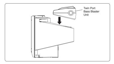
2 Firmly insert the Twin Port Bass Blaster Unit connector into the BASS SPEAKER OUT terminal.
