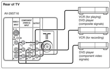
When connecting to COMPONENT (VIDEO-2) input, depending on the connection, choose the appropriate video input using the menu (see "VIDEO-2 SETTING" on page 17)
