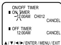
5 Press the CH + (▲) or CH – (▼) button to set the minute, then press the VOL + (▶) button.
