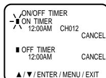
4 Press the CH + (▲) or CH – (▼) button to set the hour, then press the VOL + (▶) button.
