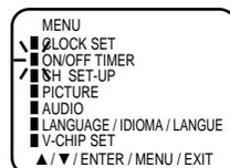
3 Press the CH + (▲) or CH – (▼) button until the indicator next to "OFF TIMER" begins to flash, then press the ENTER button.
