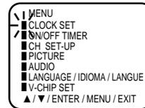
2 Press the CH + (▲) or CH – (▼) button until the indicator next to "CLOCK SET" begins to flash, then Press the ENTER button.
