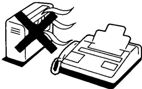
Keep the unit away from electrical noise generating devices such as fluorescent lamps and motors.
