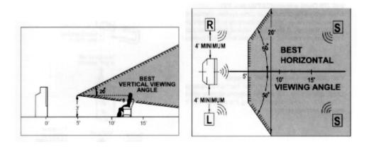
**CAUTION:** The magnetic field of external speakers may cause the TV picture to distort if the speakers are placed too close to the television. Move the speakers away from the TV until there is no picture distortion.
