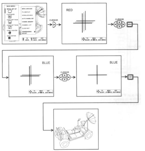
Press the CURSOR ▲ or ▼ to move the color displayed up or down. Press CURSOR ◀ or ▶ to move the color displayed left or right. Press MENU to change the color. Press EXIT to quit menu.
