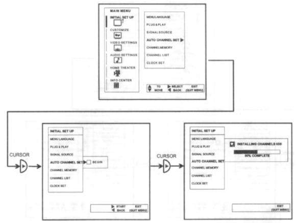
If the EXIT button is pressed while the AUTO CHANNEL SET function is engaged, programming will stop. If two antennas are connected, switch antenna inputs with the INPUT button and repeat AUTO CHANNEL SET for the second antenna input. Remember to select the correct SIGNAL SOURCE mode before using AUTO CHANNEL SET for the second antenna input.
