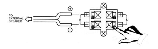
**CAUTION:** Do not connect Speakers simultaneously to the REAR SPEAKER terminal of the Projection TV and an external amplifier. This could damage both the TV and the speakers. Your TV was designed to use 8 Ohm speakers only. Any other type may degrade the audio performance of your entertainment system.
