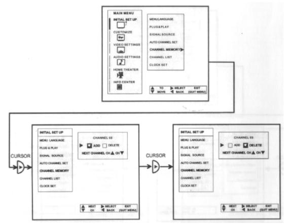
Add or erase additional channels while still in CHANNEL MEMORY using CURSOR  $\blacktriangle$  or  $\checkmark$ , CHANNEL  $\bigstar$  or  $\checkmark$ , and number buttons and then add or erase using the CURSOR  $\blacktriangleright$  button.
