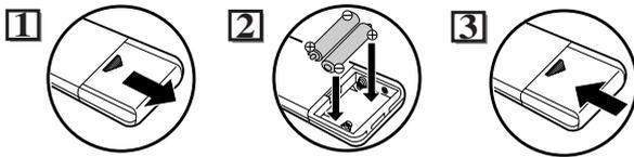
Install two AA batteries (supplied) matching the polarity indicated inside battery compartment of the remote control.
