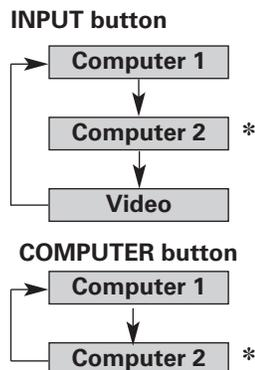
\* Computer 2 is not displayed when the COMPUTER IN 2/COMPONENT IN/MONITOR OUT terminal is used as Monitor out.
