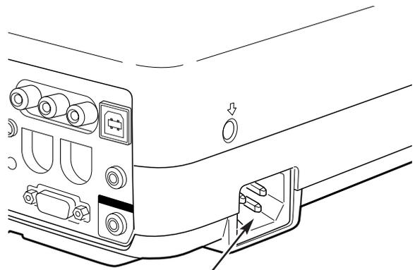
Connect AC power cord (supplied) to the projector. The AC outlet must be near this equipment and must be easily accessible.
