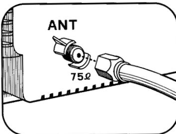
**If your cable system does not require the use of a cable box,** simply press or screw the incoming cable onto the antenna terminal on the back your TV.
