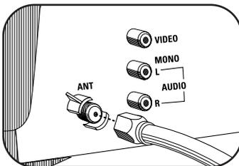
**If your cable system does not require the use of a cable box,** simply press or screw the incoming cable onto the antenna terminal on the back of your TV.
