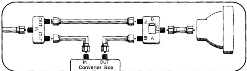
When the A/B switch is in the A position, you need to change channels on the converter box (and your TV should be tuned to channel 3 or 4); when the A/B switch is in the B position you can change channels on the TV.
