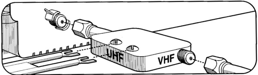
**If your antenna system has two sets of twin 300-ohm leads,** you must obtain a combiner (available at your local electronics store). Place one set of twin leads underneath the screws on the combiner and tighten the screws. Do the same with the other set of twin leads. Press the cable from the combiner onto antenna terminal on the back of your TV.
