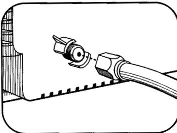
**If your cable system does not require the use of a cable box,** simply press or screw the incoming cable onto the antenna terminal on the back your TV.
