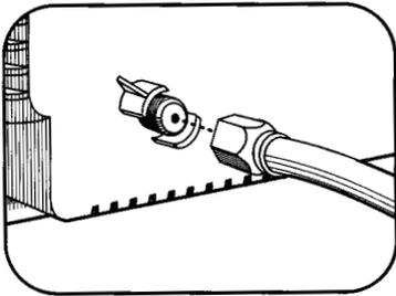
**If your antenna ends in a single coaxial lead,** simply press or screw the cable onto the antenna terminal on the back of your TV.
