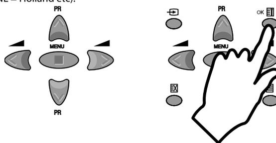
Selection is made by use of the remote control CURSOR UP (A6) / CURSOR DOWN (A21) keys and CURSOR RIGHT (A20) / LEFT (A7) keys.
