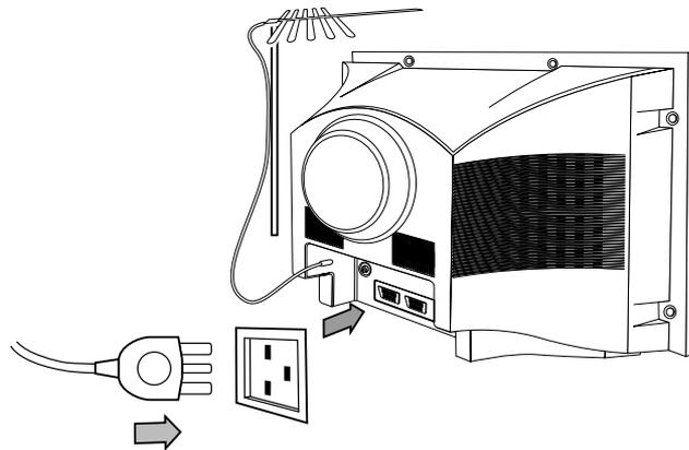
Insert the main plug into a 230V 50Hz AC power socket.
