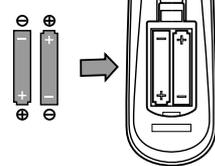
Open remote control battery compartment (at the rear) and insert two 1.5V type AAA batteries. Warning: be careful to respect battery polarities.
