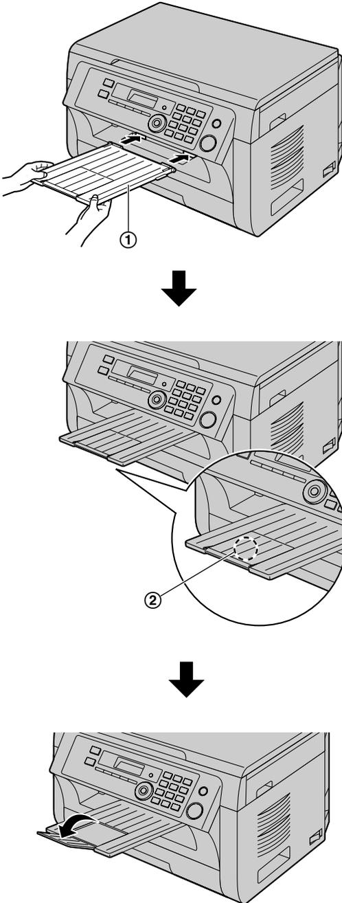
vary depending on the usage environment). Remove the printed paper before the output tray becomes full.
