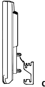
2. To secure the panel, slide forward the locks on both sides of the mounting plate. Lock the panel with one screw at both sides (D).
