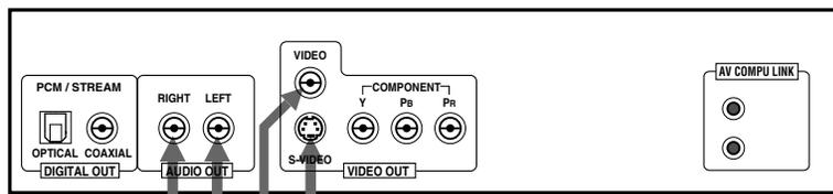
If the TV has an AV COMPU LINK terminal, you can use the AV COMPU LINK function. See "AV COMPU LINK remote control system" on page 51 for details.
