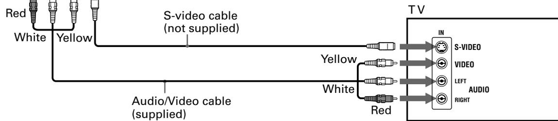
Connect the unit to a TV equipped with stereo audio input and video input jacks using the supplied audio/video cables.
