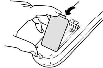
**2** Place the two accessory R6P (SUM-3)/AA(15F) batteries in the remote control according to the polarity markings (“+” and “-”) inside the compartment and on the batteries.
