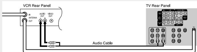
If you have a “mono” (non-stereo) VCR, use the Y-connector (not supplied) to hook up to the left and right audio input jacks of the TV. If your VCR is stereo, you must connect two cables.
