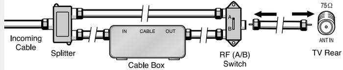
After you've made this connection, set the A/B switch to the "A" position for normal viewing. Set the A/B switch to the "B" position to view scrambled channels. (When you set the A/B switch to "B," you will need to tune your TV to the cable box's output channel, which is usually channel 3 or 4.)
