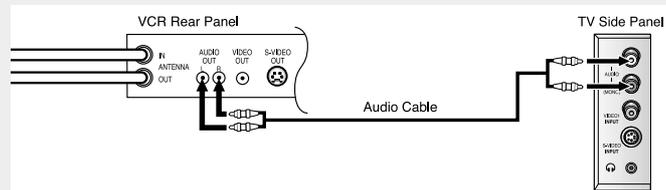
Make sure the jacks you are using are underneath the number “1.”
