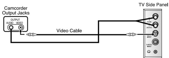
The audio-video cables shown here are usually included with a Camcorder. (If not, check your local electronics store.) If your camcorder is stereo, you need to connect a set of two cables.
