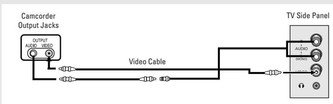
The audio-video cables shown here are usually included with a Camcorder. (If not, check your local electronics store.) If your camcorder is stereo, you need to connect a set of two cables.
