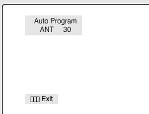
◀ The TV automatically cycles through all of the available channels and stores them in memory. This takes about one to two minutes. Press the **MENU** button at any time to interrupt the memorization process and return to the Channel menu.
