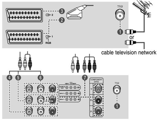
⚠ Whenever you connect an audio or video system to your television, ensure that all elements are switched off. Please be sure to match the color coded input terminals and cable jacks.
